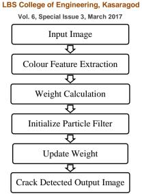
Fig.2. Block diagram of the crack detection method
